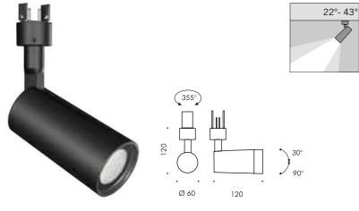
S.9020W From Medium to Flood beam with lens LED MODULE 3000K CRI90 852Im 8,6W (on request 2700K CRI90 807Im) (on request 4000K CRI80 1056lm) Rated input power 9,5W 24Vdc PWM
