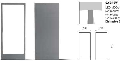
LED MODULE **3000K** CRI90 5250Im 44,5W (on request 2700K CRI90 3686Im) (on request 4000K CRI80 6090Im) 220V-240Vac 50/60Hz **Dimmable DALI 2 / PUSH**
