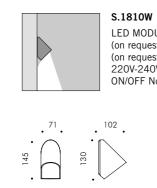
LED MODULE **3000K** CRI90 1342Im 12,5W (on request 2700K CRI90 1246Im) (on request 4000K CRI80 1658Im) 220V-240Vac 50/60Hz ON/OFF Not Dimmable
