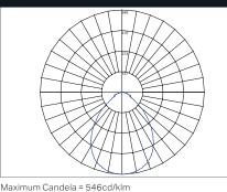
Maximum Candela = 546cd/klm Located At Horizontal Angle = 90, Vertical Angle = 1
