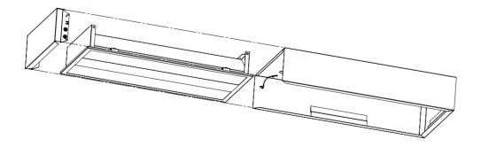
\* Please ensure a minimum clearance between the luminaire and vertical wall is greater than the length of the luminaire
