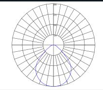
Maximum Candela = 496cd/klm Located At Horizontal Angle = 67.5, Vertical Angle = .5
