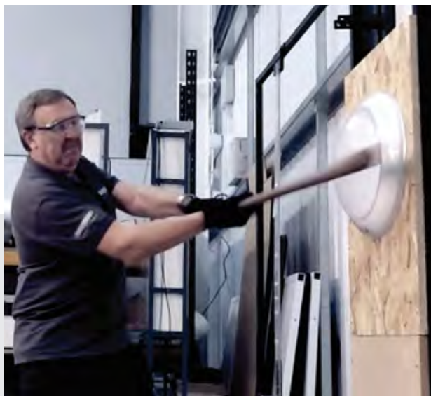
IK TESTING: Measuring impact resistance
