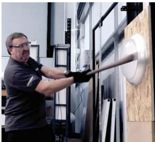
IK TESTING: Measuring impact resistance
