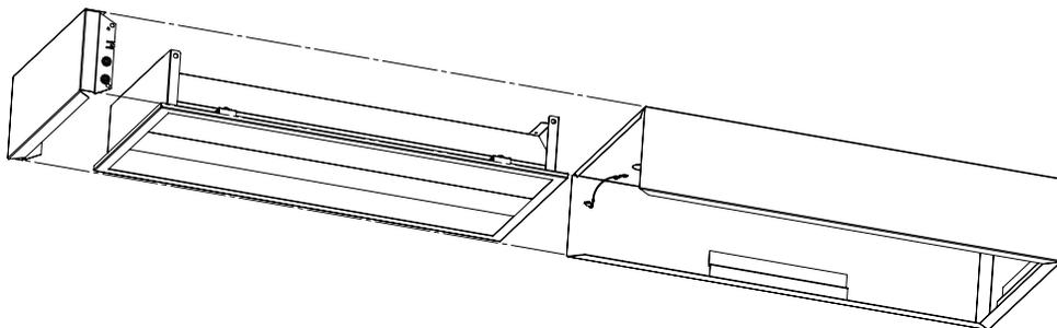
\* Please ensure a minimum clearance between the luminaire and vertical wall is greater than the length of the luminaire
