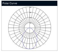
Maximum Candela = 546cd/klm Located At Horizontal Angle = 45, Vertical Angle = .5
