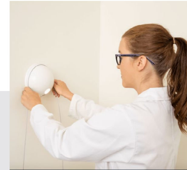
LIGATURE RESISTANCE TESTING: Ensuring safety against self-harm
