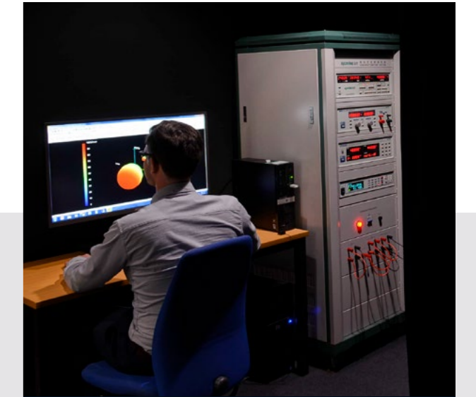
PHOTOMETRIC TESTING: To measure light performance
