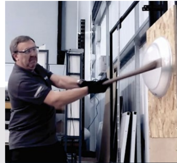
IK TESTING: Measuring impact resistance
